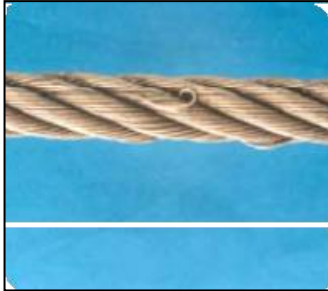
Damaged steel wire rope
