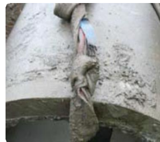
Fibre slings with knots
