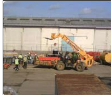
Attachment and load incorrectly positioned
