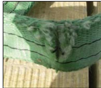
Sling damaged on sharp edges
