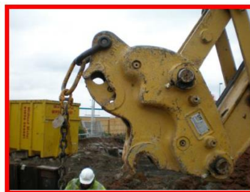
Figure 4. – Hitch tilted backwards with master link subject to twisting
