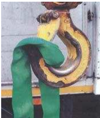
Conventional Safety Hook with Continuous Webbing Sling
