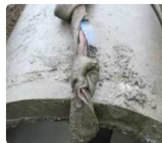
Fibre slings with knots
