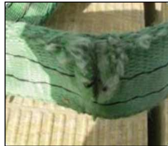
Sling damaged on sharp edges
