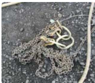
Badly stored chain slings
