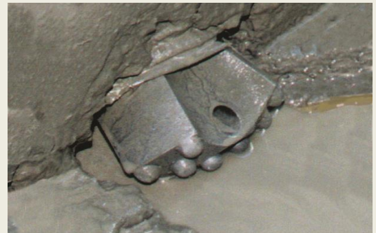
BUTTON BIT CAN DRILL THROUGH CONCRETE
