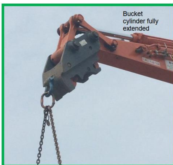
Figure 5. – Chain and master link can hang freely without obstruction (Note Bucket Cylinder is fully extended, if the load needs to be rotated then a swivel is required as in Fig.2)
