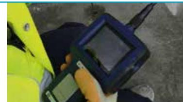
Endoscope inspection of anchor ring
