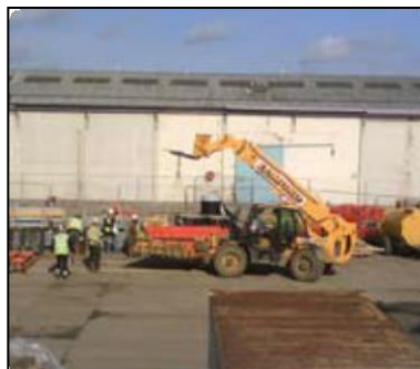
Attachment and load incorrectly positioned
