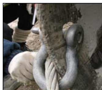
Shackle pin not flush with shackle – it must be 'finger tight'
