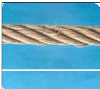
Damaged steel wire rope
