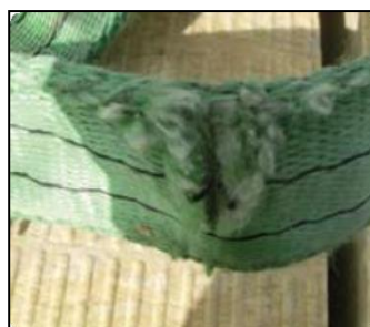
Sling damaged on sharp edges
