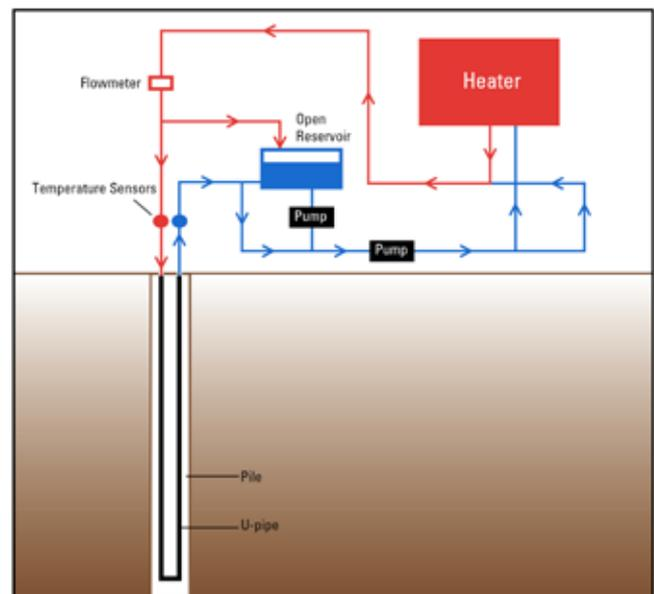
to the heating or cooling available measured in W/m/K. A thermal response is carried out using a self contained portable test unit towed behind a 4 x 4 vehicle. A properly conducted test will take 3 to 4 hours to set up and then 3 to 4 days to complete. Analysis of the results and reporting can then take place.
